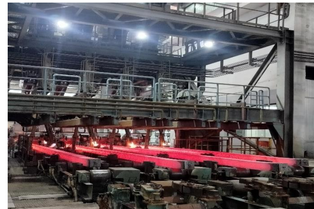
Billet Caster in SMS-2 at BPSL
